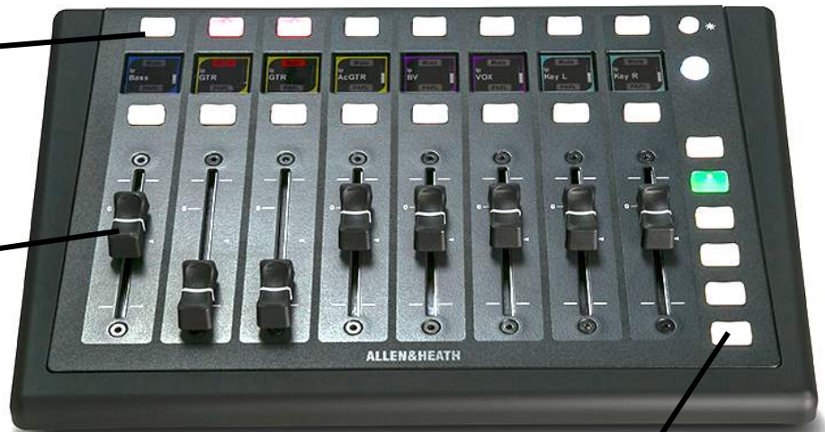
IP8 (Theatre Controller)
